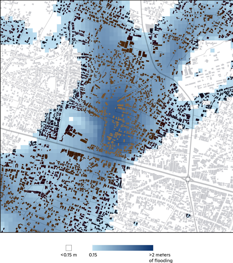
Figure A5: Flood inundation map for a 1-in-100 year rainfall event for 2041–2060 with building polygons included.
