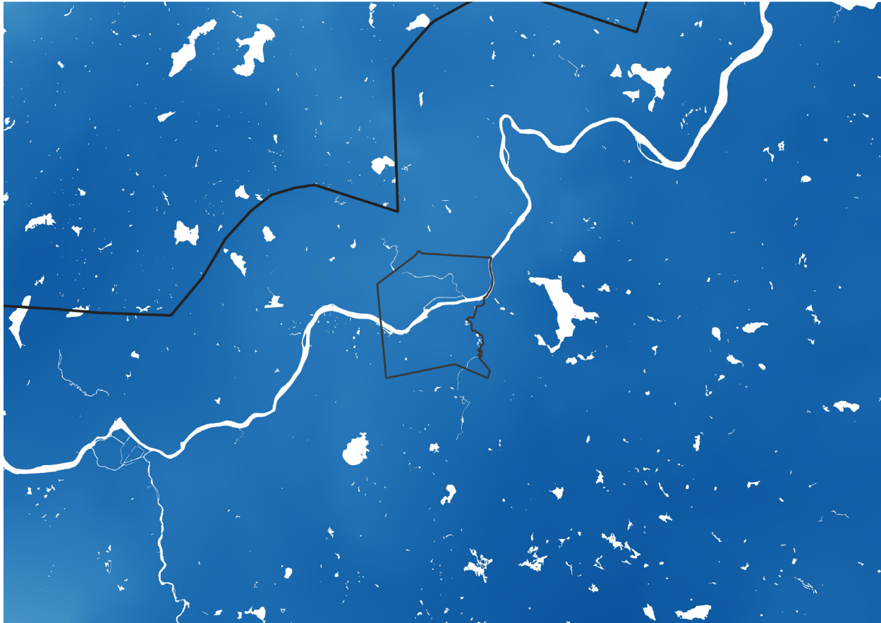
Figure 2: Late-21st Century Change in Historical 100-Year Rainfall. The future return period of the 2000–2020 100-year rainfall event in 2070–2090 with the darker the blue, the smaller the return period (greater frequency of occurrence). By the late 21st century, the historical 100-year rainfall event is expected to become a 1-in-10 to 1-in-15 year event for much of the Merrimack River valley.
