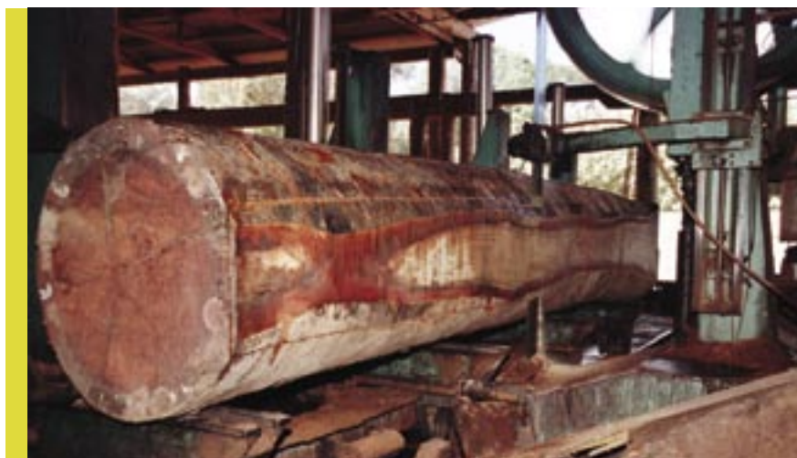
Sawmill technology in the Amazon (such as the bandsaw shown here) has not changed much since the 1950s. Efficiency is between 30 and 40 percent yield from log to boards.
