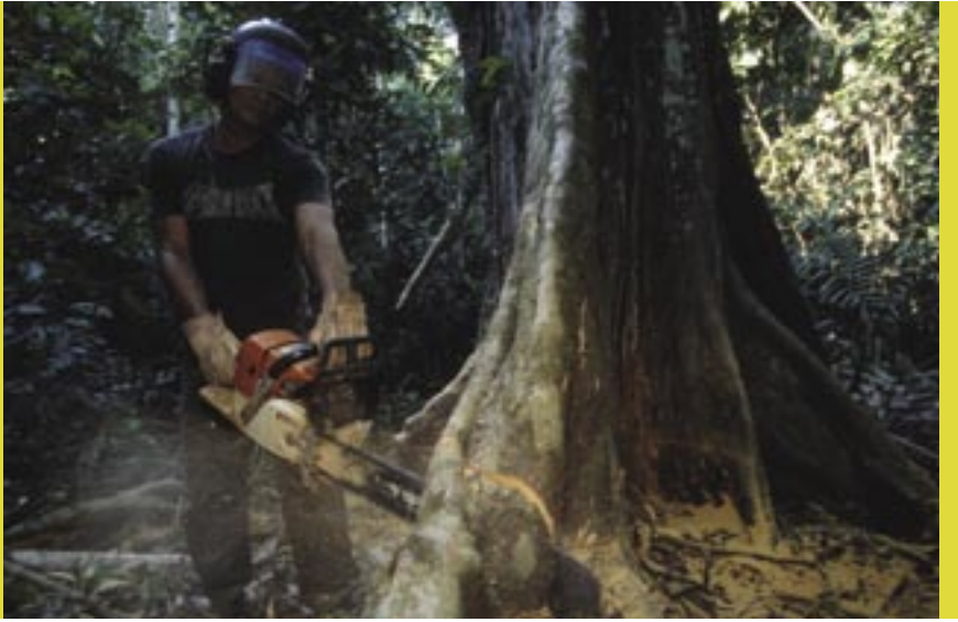
Directional felling, as shown here as part of a reduced impact logging program in the Tapajós National Forest, near Santarém, can reduce damage and help in the search for sustainability.
