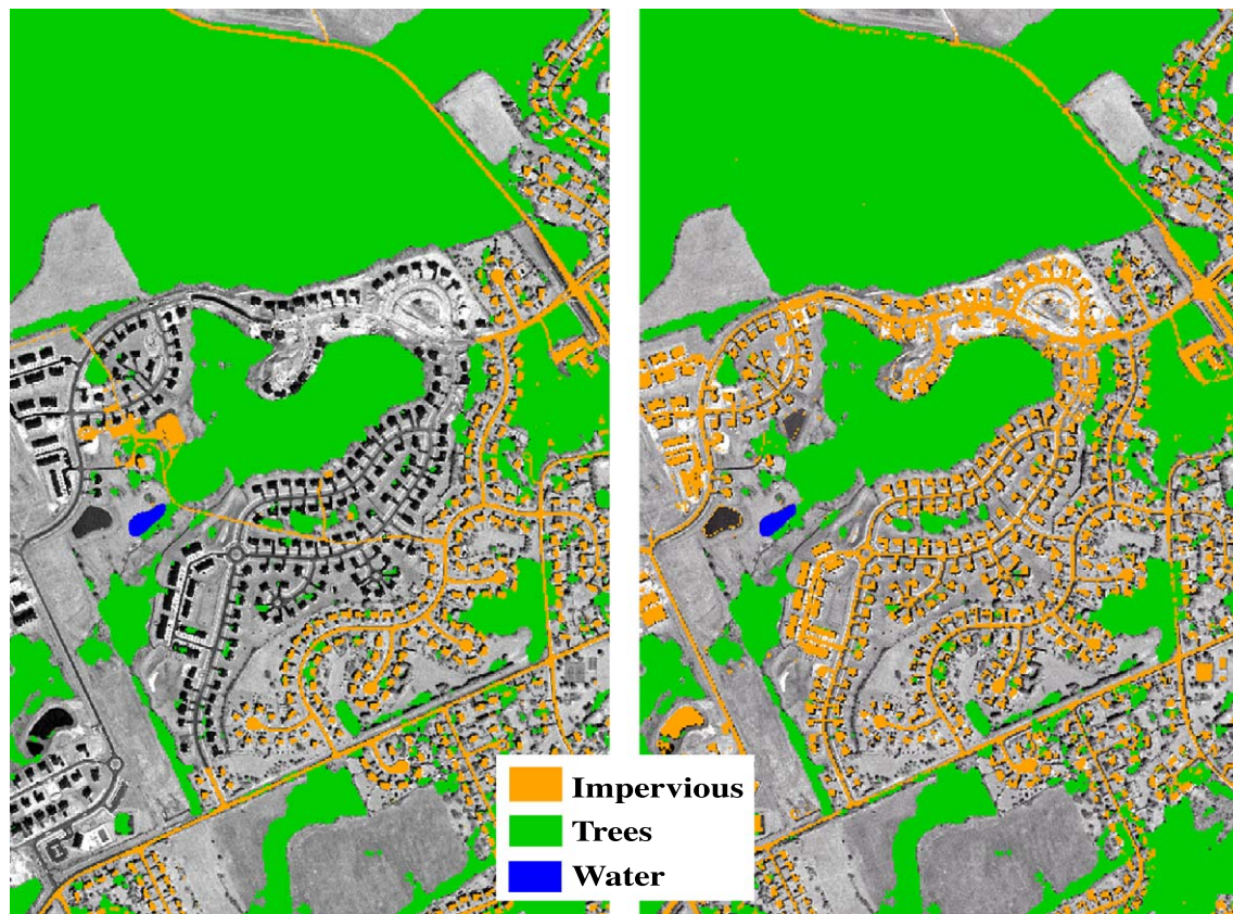
Fig. 5. Impervious surface areas (yellow) for a portion of Montgomery County derived from IKONOS imagery (right) compared to planimetric coverage derived from aerial photographs (left), showing changes in residential development since the area was initially mapped (ca. 1993). IKONOS tree cover (green) is also shown, with the IKONOS panchromatic image as a backdrop. (Includes material from Space Imaging©.)
